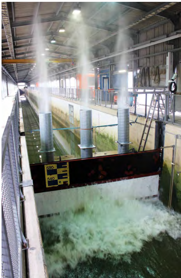
The model of a wave power plant will be tested in the large wave channel of the Coastal Research Center (FZK) in Hanover.
