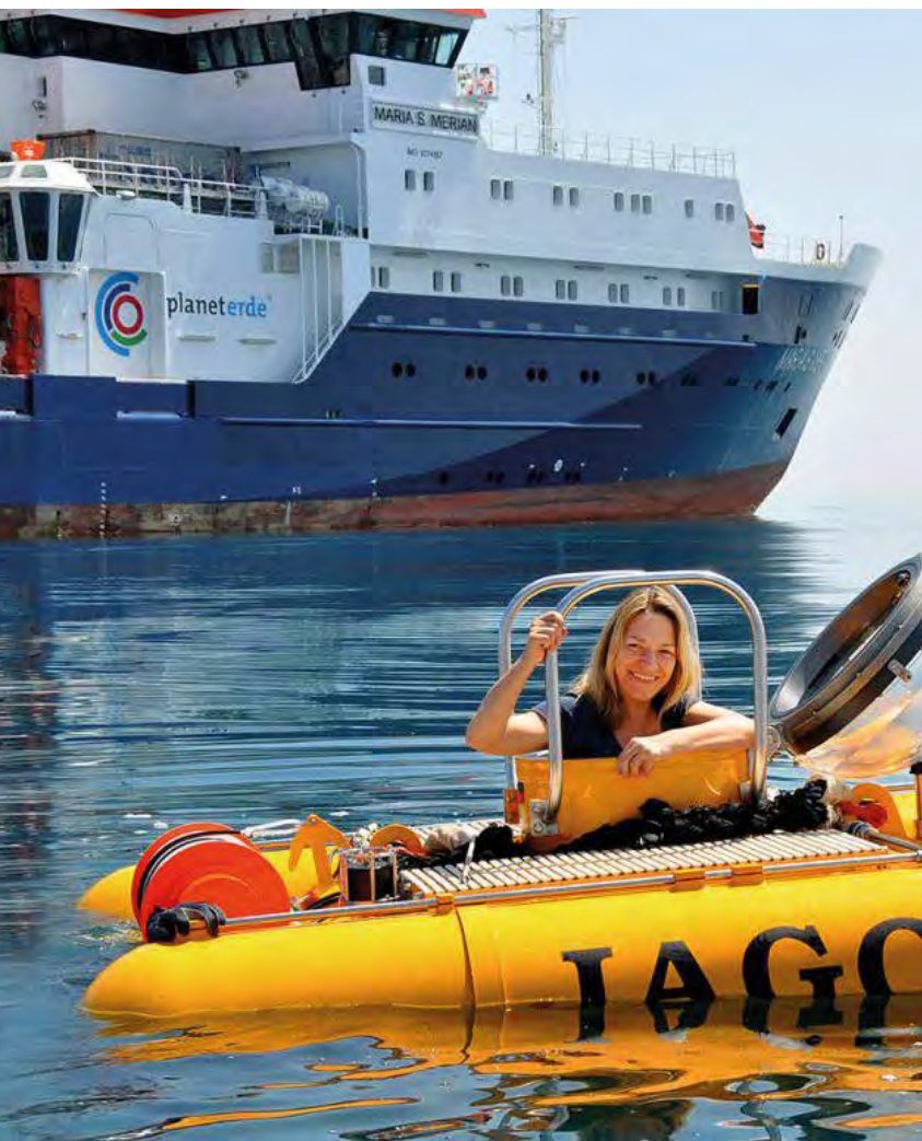
The manned underwater vehicle JAGO can dive to depths of up to 400 meters. It is used for the exploration and research of aquatic systems and habitats.
