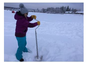
**Fig. 1 The local turn.** Dawn Pomrening, Sidney Huntington School, Galena, Alaska, measures ice thickness with the Fresh Eyes on Ice project (photo by Christopher Arp). This is an example of engaging local observers in collecting data that are of value to a broad array of scientific and forecasting applications while also integrating STEM education into the research process.
